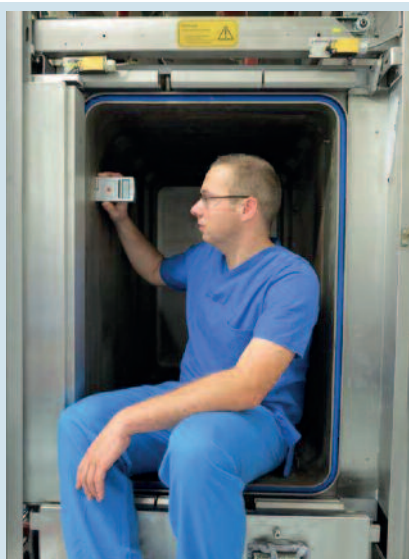
Figure 11: Quality assurance (surface roughness measurement on the chamber's interior surface) (source: Henkel Beiz- und Elektropoliertechnik)
