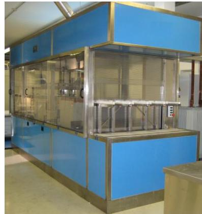
Automatic electropolishing unit for small series parts (medical technology)
