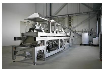
Electropolishing system for special components (basic research project)
