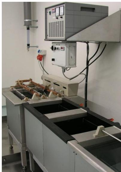
Manual electropolishing unit for small parts/components
