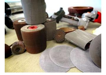
The initial grain size for coarse pre-grinding is always determined by the initial roughness of the surface and the grinding layer which is to be removed by this process. The initial grain size is generally selected on the basis that the grinding surface can reach the base of the groove and therefore that the defects (macro-defects) can be safely removed deep into the grooves.
